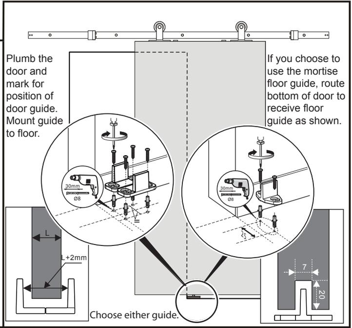
Plumb the door and mark for position of door guide. Mount guide to floor.
